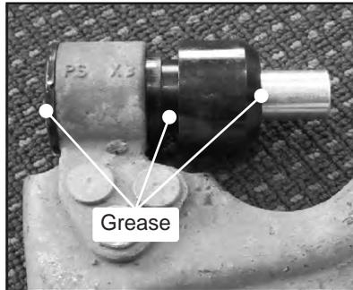
Step 1 Remove the OEM bushing by drilling a pilot hole through the rubber cushion and stepping up in drill size until the shank of the drill cuts through the outer shell.
