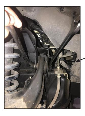
Loosen and remove the 2 inner bushing bolts.
