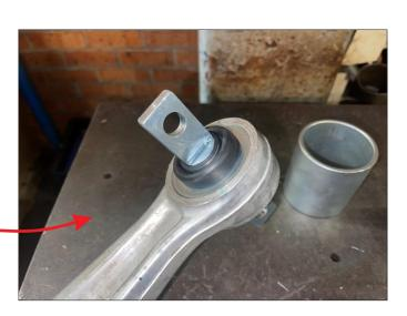
Proceed to bolt arm in vehicle with supplied reinforcement tubes and original bolts.
