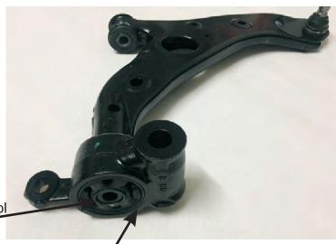
1. Place Press pressure on control arm spindle.
