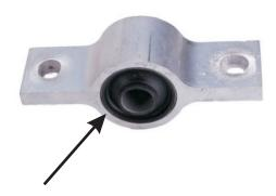
Press out OE bushing including steel outer shell
