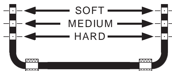
WHITELINE Blade adjustable swaybar - rate adjustment guide
