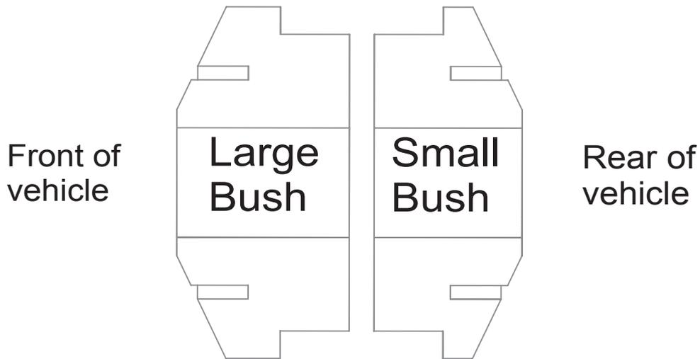
Bush is to be installed into hub with pin voiding vertically apposed.
