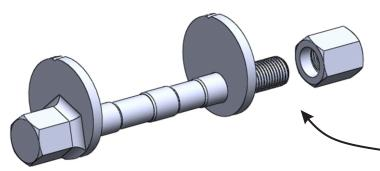
During assemble - note thread recess in nut. This should be screwed on first.
