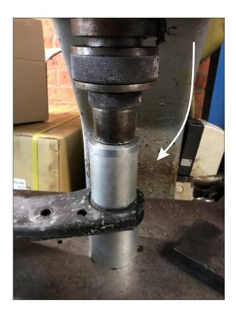
Press new bushing into arm - confirm bushing sits central in arm.
