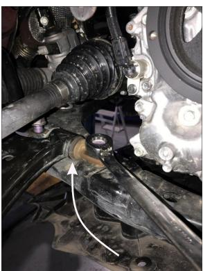
• Un-bolt rear vertical through-bolt (and nut).
