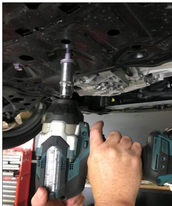
3. Start to remove the factory pit-stop by loosening the M10 bolts at gearbox,
