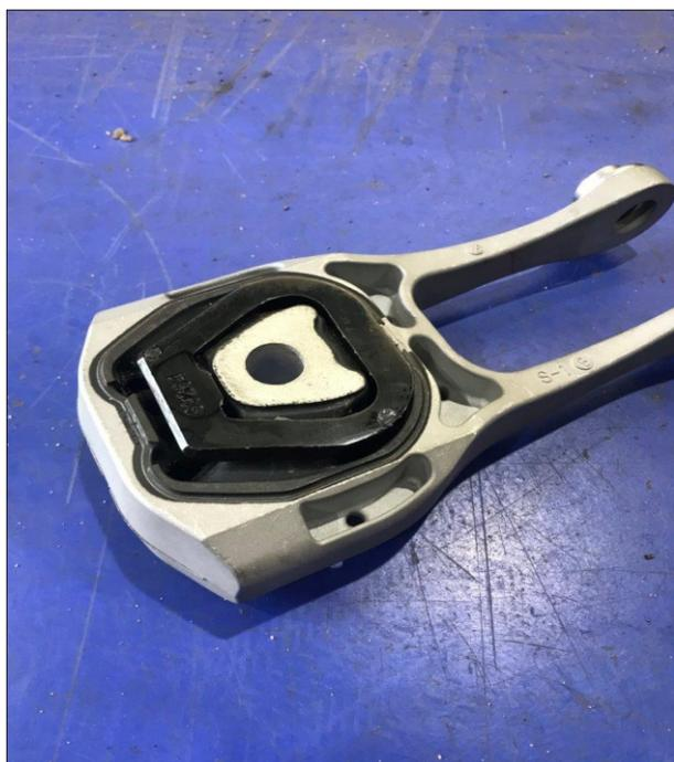
6. Re-fit mount to vehicle with original bolts. Torque bolts to manufacturers spec.
