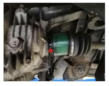
7. Remove 4 drive shaft bolts and remove drive shaft from vehicle.
