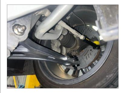
Bolt up the extended ball joint using original bolts.
