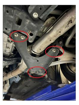
Remove the lower ball joint by loosening and removing the OE M14 nut and bolt.
