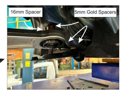
• Tighten the rear M14 bolts to 120Nm/85ft.lbs
