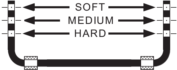
WHITELINE Blade adjustable swaybar - rate adjustment guide
