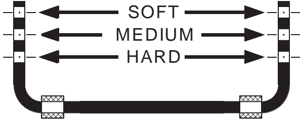
WHITELINE Blade adjustable swaybar - rate adjustment guide
