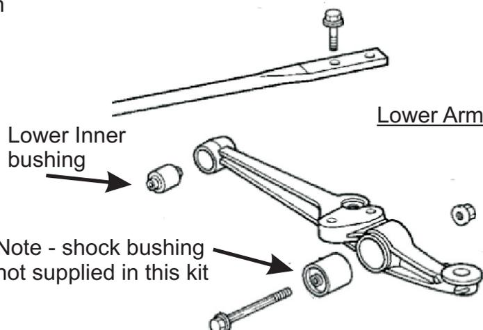
Grease bushing face and internal diameter
