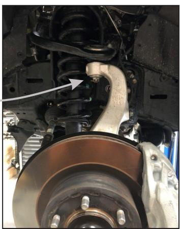
Note - check if vehicle has a head light sensor. If so, remove bracket also.
