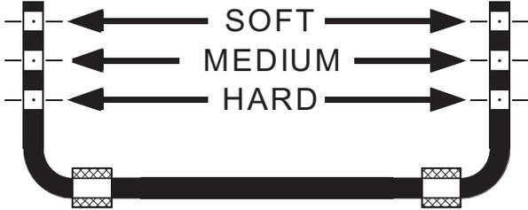
WHITELINE Blade adjustable swaybar - rate adjustment guide
