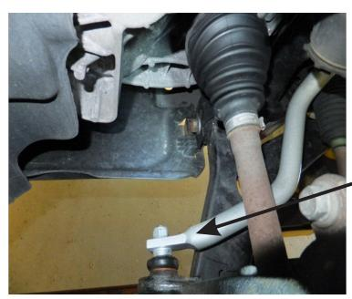
8. Once **High tensile mounting bolts** are secure, front lower control arm front bushing bolts are ball joint to hub re-installed, housing can be slid forward or backward to engage positive location on the **Flat Washer** - Large that has been installed over the spigot on the control arm. Tighten all removed bolts to manufacturers torque specifications.
