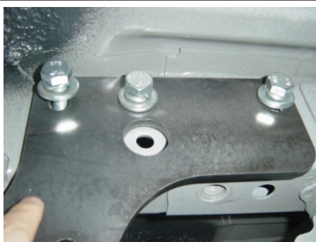
Diagram 3: Lightly secure Side Chassis Mounts (LH side Chassis Mount shown).
