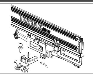
Insert head and shank assembly from step 2 into towbar hitch receiver and secure it with pull pin, and R-clip (supplied with towbar).
