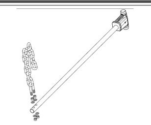
Ensure M10 U-bolts (item 12) & M10 nuts (item 14) in both spring bar assemblies are loosely assembled to the same height position.
