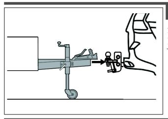
Attach trailer coupling to the towball mount as shown. Ensure coupling is fully engaged and remove load from jockey wheel.
