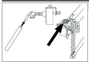
Insert extension handle (item 6) onto tension lever clamp. Open tension lever clamp until arm is parallel to the ground. Lift chain by hand and hook onto tension lever clamp arm. Using both hands raise tension lever clamp arm to final position. While firmly holding in final position insert locking pin (item 11).
