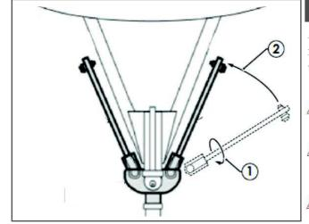
Attach both spring bar assembles into the LDH head by first rolling the spring bar in the head and then moving it inboard to align with trailer A-frame.
