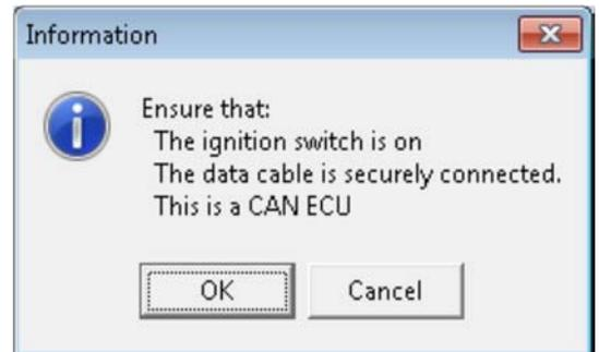
Sometimes the CAN bus can time out (especially after a communications error – on Subaru CAN models the temp gauge on the dash will flick straight to High), in which case simply turn the ignition off, then turn it back on and try again.
