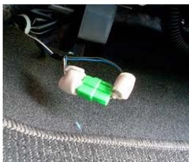
If you have found and connected these correctly, when you turn the ignition on (but don't start the engine) the Check Engine Light on the dash will flash. At this point, hit "Enter Utility Mode" on the laptop and follow the directions on screen. To complete entry into Utility Mode you will need to leave the ign ON and disconnect the green connectors as directed.
