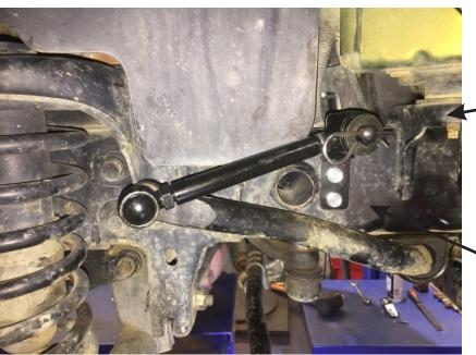
Bolt chassis pin up to chassis bracket using 3/8 nut flat washer.
