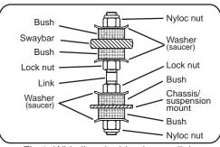
Fig.1. Whiteline double pin type link.
