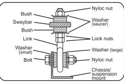
Fig.2. Whiteline pin/eye type link.
