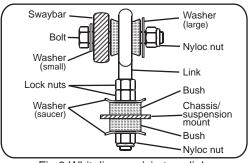
Fig.3 Whiteline eye/pin type link.
