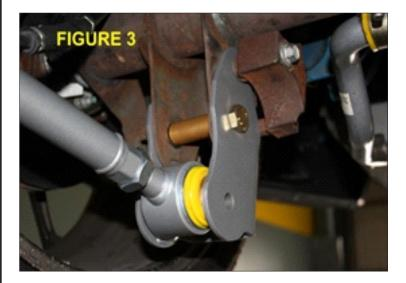
• Position arm in the lower hole and insert the 100mm bolt with the nyloc nut on the outside facing the wheel. Positioning may require use of pry bar. Tighten bolt to 129 ft/lb
