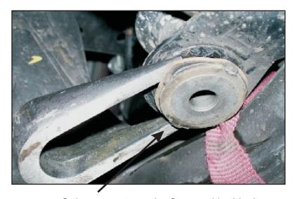
Gain access to under flange with chisel
