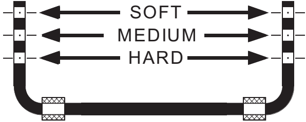
WHITELINE Blade adjustable swaybar - rate adjustment guide
