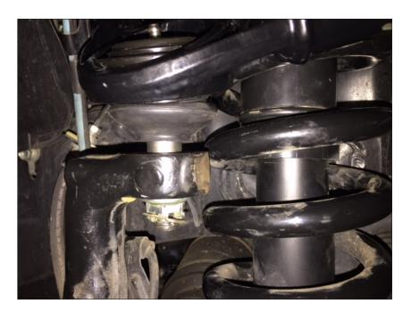
• Connect ball joint to hub - and tighten with flange nut.
