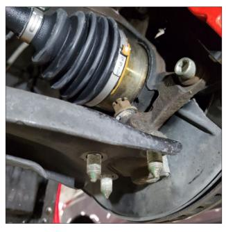
Remove Ball Joints from vehicle.
