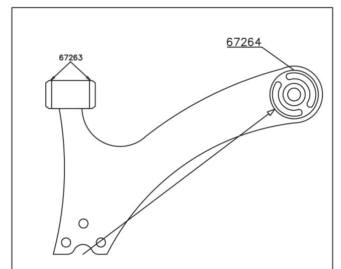
place voiding inline with ball joint as indicated by arrow.
