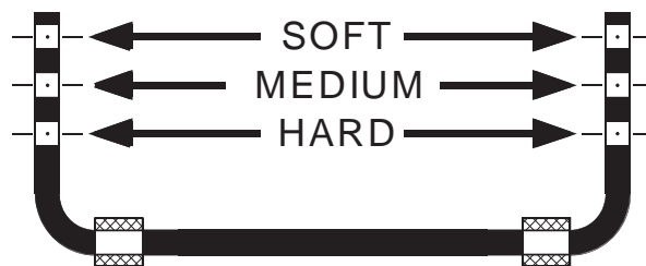
WHITELINE Blade adjustable swaybar - rate adjustment guide
