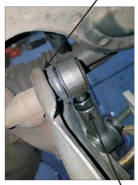
Tighten lock nut when desired \ length is achieved - note minimum thread engagement is 15mm
