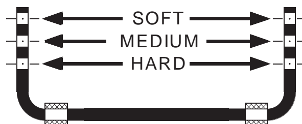
WHITELINE Blade adjustable swaybar - rate adjustment guide
