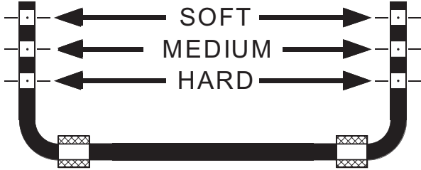
WHITELINE Blade adjustable swaybar - rate adjustment guide
