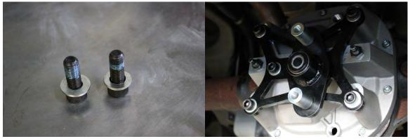
18. Remove the upper support brace located just above the Panhard bar location, using a 15mm socket for the two driver side bolts and an 18mm for the passenger side. Keep the fasteners as they will be re-used later.
