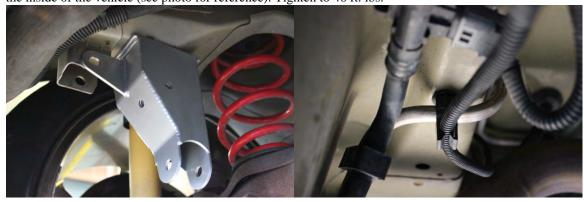
20. Directly above the differential there are 3 lines for the fuel system held by a retainer clip, it is required to flip the direction of this clip to allow clearance (see below), remove the secondary single retainer clip (see above).
