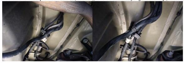
21. Using the supplied vinyl clamp and self-tapping screw, secure the fuel line to the chassis, then zip tie the wiring harness to it as shown below. This will replace the removed plastic clip.
