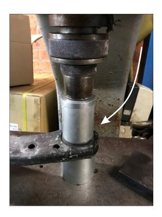
Note - bushing diameter is 55mm U.se a Press Tool 53-54mm in diameter. P/No PKN06.
