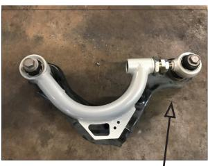
Prior to bolting arm up to vehicle, place the OE bolts through both bushings as per above. Place WHITELINE arm over OE arm - to pre-set length.
