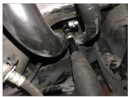
The inner point is difficult to get to on the LH side. Use a 3/8 ratchet to access M12 bolt.
