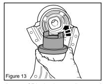
13. Install the 9170B bush into the bottom of the rear lower cradle mount OE bush using a small amount of grease supplied. (Figure 13 & Figure 14).
