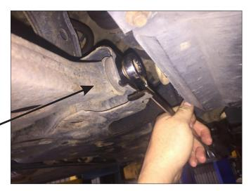
• Un-bolt front bushing bolt. Note - for RHS, loosen and lower A/C compressor gaurd to remove bolt.
