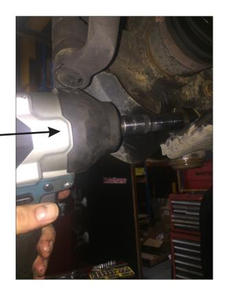
• Un-bolt rear bracket from sub-frame.
