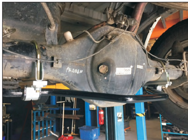
Axle mounting components - U bolts Axle brackets Flat plates D Saddle Flange nuts
