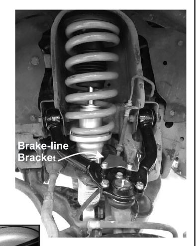
Using original bolts, bolt up ABS wire bracket under arm
