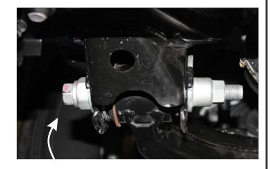
Note - the front bushing needs to be loosened via the bolt head, not nut
