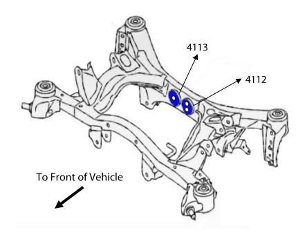
Note: It is possible to remove and replace these bushes without removing cross member
