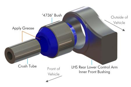
Figure 02 - '4736' bushing installation
