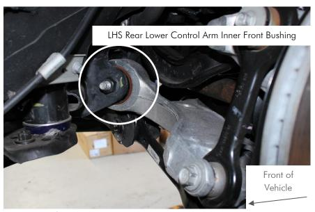
Figure 01 – Left Hand Side Lower Control Arm Inner Front bushing
