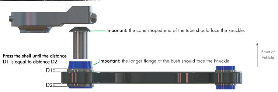
Figure 03 – Left Hand Side Upper Control Arm Outer Bush Installation
