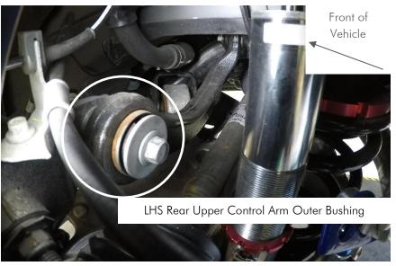
Figure 01 – Left Hand Side Upper Control Arm
