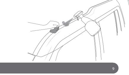
(A) Using butyl mastic, apply the sealant to all exposed holes in the roof.(B) Add 2x butyl patches to these holes in the roof.
