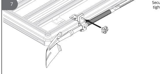
Secure the carried item by tightening with the plastic knobs provided.
