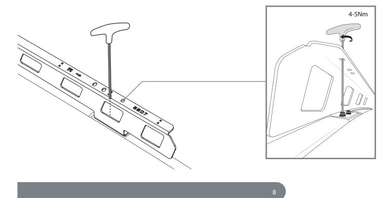
Assemble the stud plates and corresponding hardware onto the system. Tighten in place.
