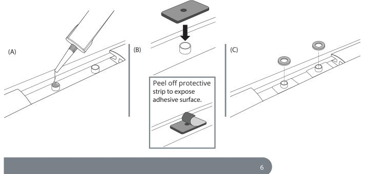
Assemble M8 hardware into the Ridge Mount rails as shown.
