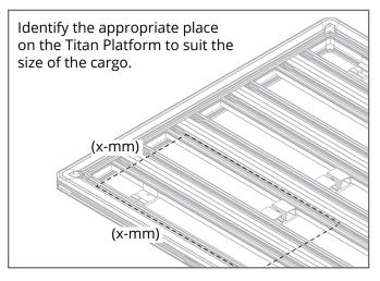
Slide a T-bolt into the c-channel of the platform, moving them to dimensions of the previous step.
