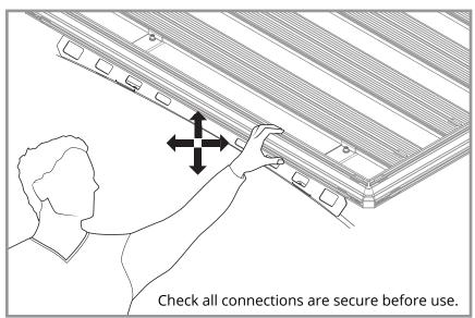
Wiring can be run and secured on the underside of the Ridge Mount rail as shown.
