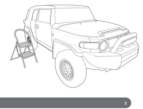
Carefully remove the 6 mounting point covers from the roof.
